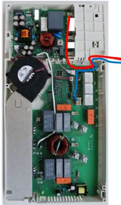
2-burner slave generator (left)
