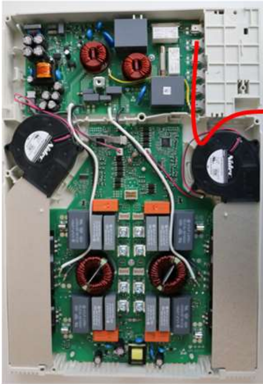
4-burner master generator (left)
