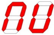
Figure 7: Indication of bridge function “master” and “slave” cooking zones on 7-segment display
