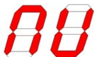
Figure 9: Indication of bridge function “master” and “slave” cooking zones on 7-segment display
